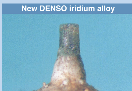
Test engine: 90 cc 4-cycle 1-cylinder Test conditions: Fullx9000rpmx30h
