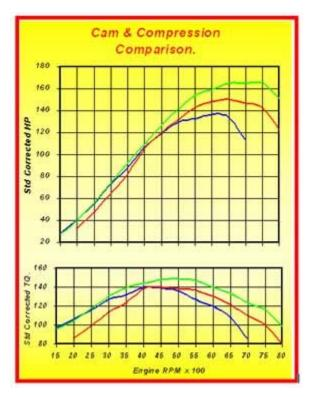
CR. The biggest gains seen were at the low end. With 11.5/1 the motor could be pulled down to 1500 rpm where it made only 1.5 lbs.-ft less torque than the stock cam/compression combination. By pairing the cam duration with an appropriate CR peak power increased by 26 hp with virtually no low speed penalty.
