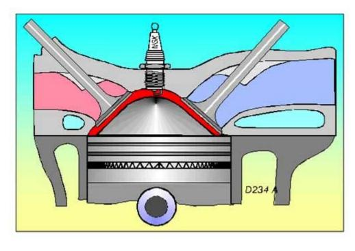
The last points that we will discuss here concerning combustion chambers relates to the chambers compactness. The fact that ultra high CR's are being sought means the object of the exercise is maximum power. This also infers the need to turn maximum rpm. If so short stroke/big bore motors look
