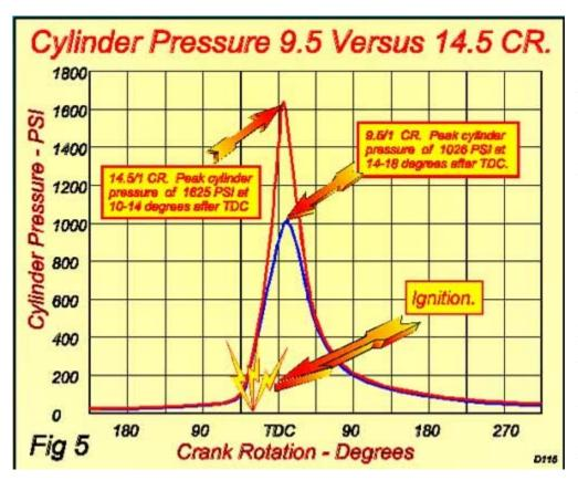
When the compression ratio is raised peak cylinder pressures follow suit. A basic rule of thumb is that peak pressures will be approximately 100 -110 p.s.i. for every ratio. A 10/1 ratio motor will typically see 1000-1100 p.s.i. peak pressure. A 16/1 motor will be between 1600 and 1760. An ultra high CR then means big pressure numbers. This
