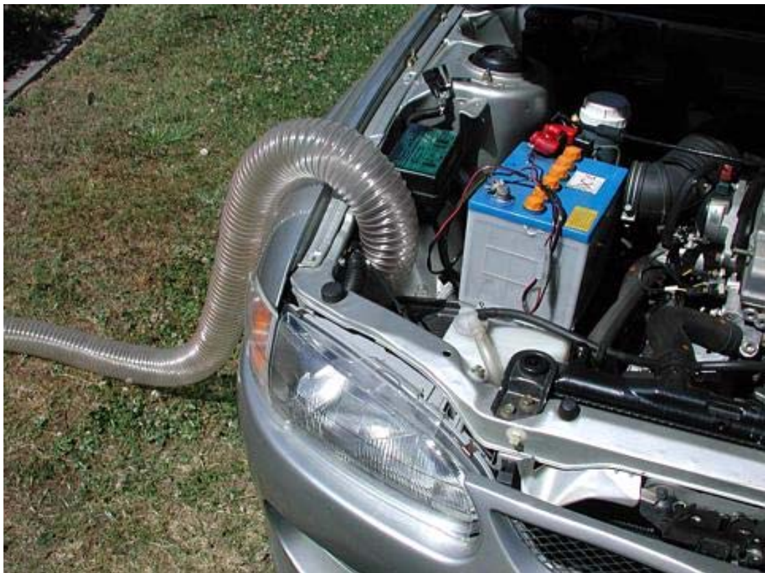
5. SPEEDFLEX SFS 82 HOSING Feeding from the top is best and cut to length.
