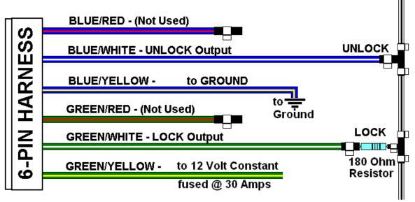
NOTE \*\*\* Connect the BLUE/YELLOW wire to a GROUND and the GREEN/YELLOW wire to 12 Volt Constant and fuse @30 Amps
