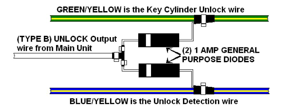
These wires are located in a Plug below the Fuse Box.
