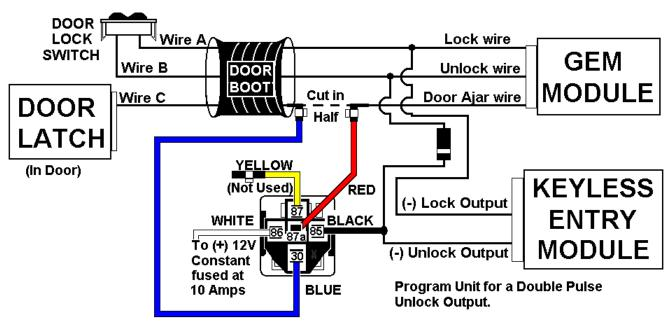
NOTE: When testing the DOOR AJAR wire, it will rest at (-) Ground when the door is closed and pulse to (+) 12V when the door opens, then returns to (-) Ground. This Diagram will also activate the Dome Light when Unlocking
