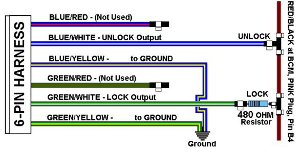
NOTE \*\* Attach the BLUE/YELLOW and the GREEN/YELLOW wires to a SOLID BODY GROUND.
