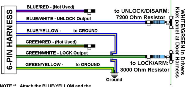
NOTE \*\* Attach the BLUE/YELLOW and the GREEN/YELLOW wires to a SOLID BODY GROUND.
