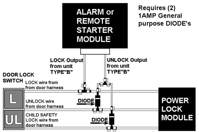
The CHILD SAFETY LOCK wire is in the same door harness as the LOCK and the UNLOCK wire in the DRIVERS KICK PANEL.
