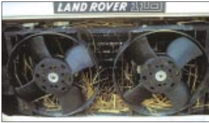
Above: The result of no radiator protection in tall grass.
