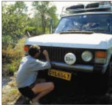
Fine aluminium mesh is the best material to use for a grille net as it allows good air flow while preventing the passage of seeds and grass.
