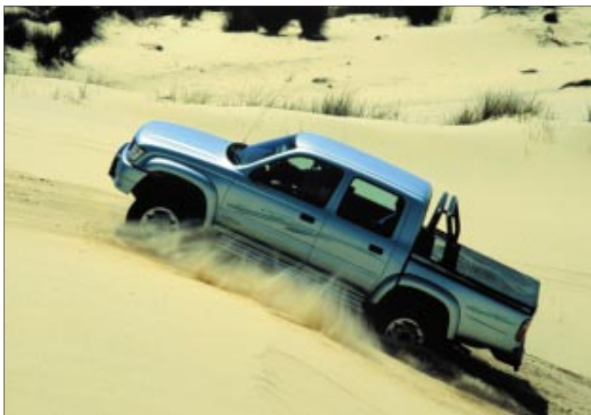
The secret of safe dune driving is establishing momentum at the base of the slope and then correctly timing the deceleration at the summit.
