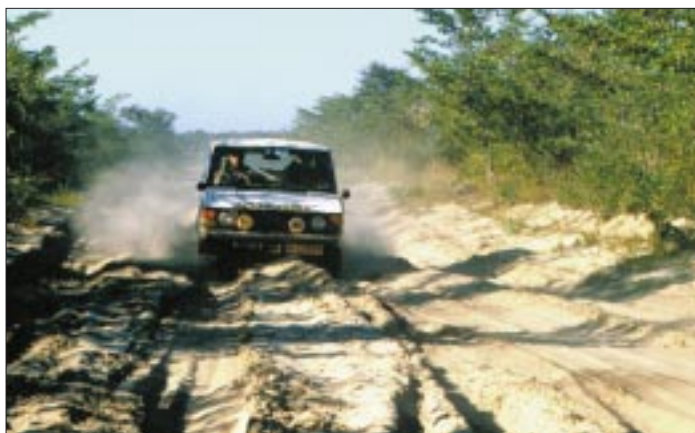
Sand tracks in the Kalahari. Engage 4WD or lock the centre diff even if you don't think you need it.
