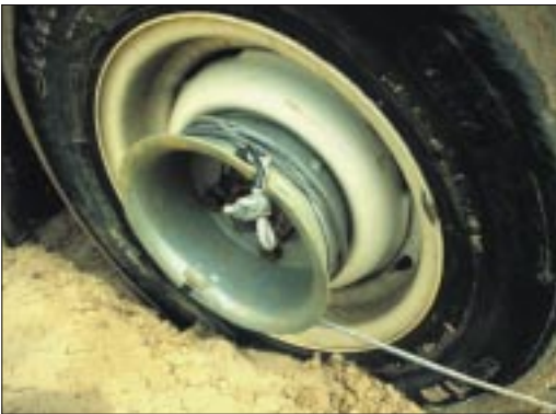
Left: A hub capstan winch attached to a Land Rover Defender's standard steel rim. Lightweight, practical and cheap, it is unfortunate that hub capstans are not available for a wider range of vehicles.
