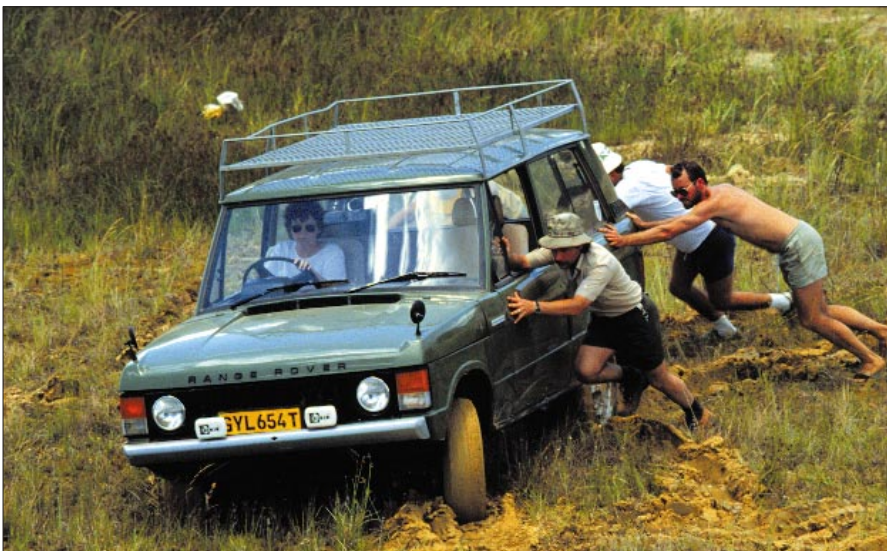
Always consider a push - its quicker to organise than a winch or tuggum.
