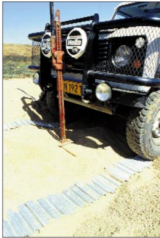
Jack & Pack - lift with the high-lift and then lay sand tracks under the front wheels.
