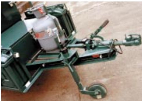
Equipment on the draw bar must not be too far forward. Check that the tailgate can be opened with the trailer hitched on.
