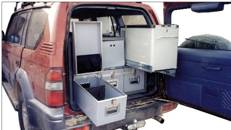
Primary containers can be compartmentalised for convenience and can be made from expensive 'camera case' aluminium or painted steel plate.
