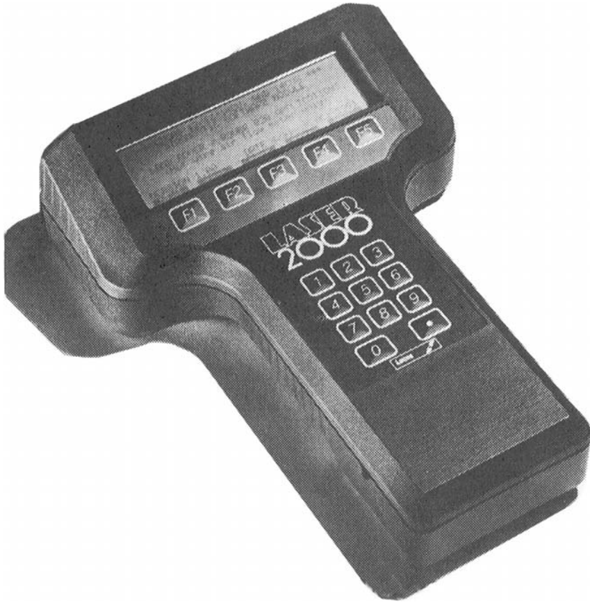
Fig. 4.1 Laser 2000 uses the on-board diagnostic facilities incorporated in the ECU's controlling vehicle systems. The sophistication of these facilities varies considerably across vehicle manufacturers
