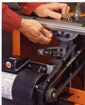
Adjusting blade alignment. A cam and lever on the rear trunnion make it easy to align the blade to the miter-gauge slot.
