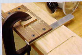
A straightedge for more than layout. The 1/4-in.-thick aluminum blades also can be used as a fence for short router cuts.
