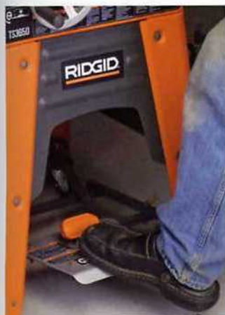
Retractable casters. A foot pedal controls a scissors lift that activates four retractable rubber wheels.
