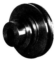
Fig. 1. The finished pulley
