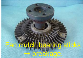
Cracks appear at the Fan diagonally
