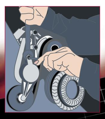
Always check the condition of the automatic tensioner. If it is not functioning properly, replace it with a Gates DriveAlign<sup>®</sup> tensioner. For more information on Gates DriveAlign<sup>®</sup> tensioners, please consult leaflet E2/70380 or catalogue E/70378.
