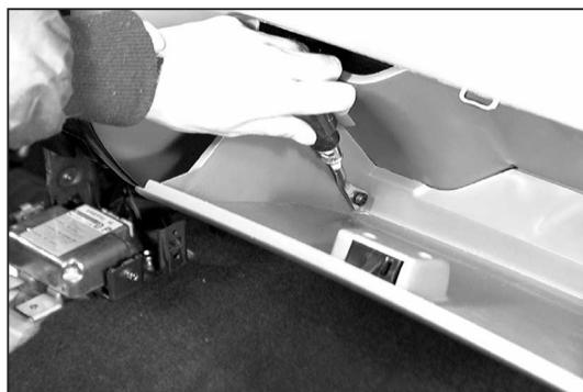
12. Removal of instrument cluster finish center panel assembly
