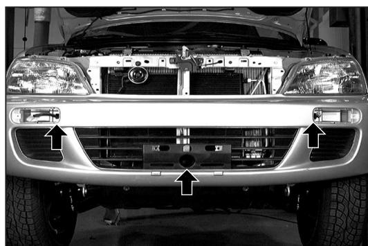
5. Remove the attaching bolts of the front bumper cover. (On model without the front bumper guard garnish.)
