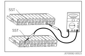
(4) Temporarily connect a vacuum gauge (The MityVac may be used) to the negative pressure port of the VSV so that the inner pressure of the intake manifold may be measured. Next, start the engine and keep it idling. At this time, ensure that the gauge reading and the voltage across the SST terminals 24 and 52 satisfy the following formula given below.
