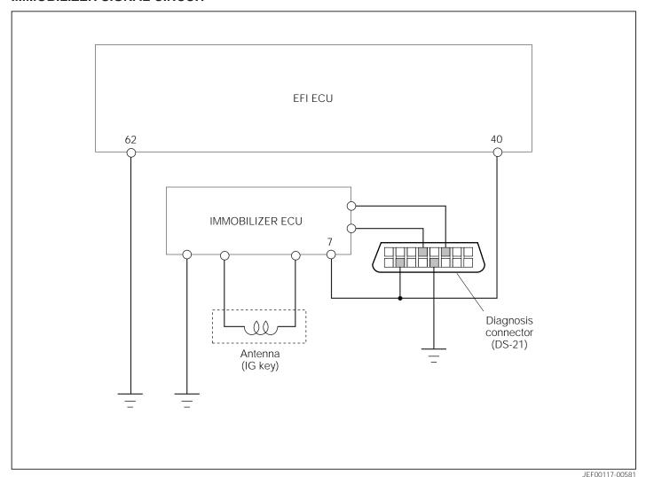
When the rolling codes cannot be exchanged between the engine EFI ECU and the immobilizer ECU or the rolling codes are not matched.
