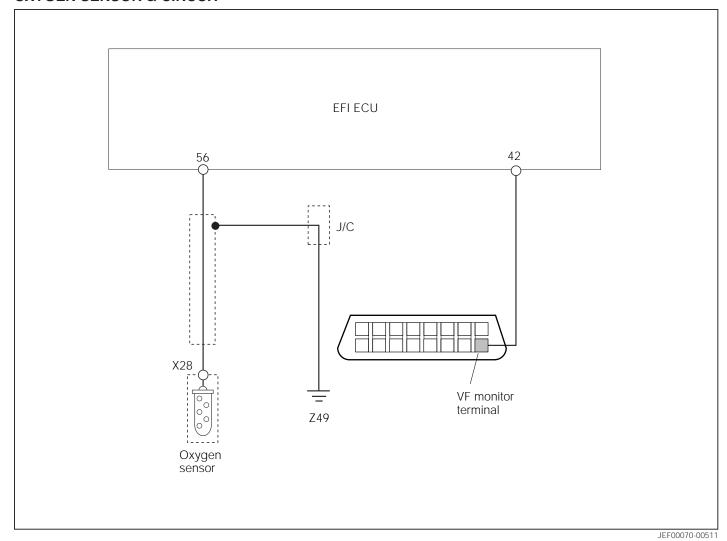
The ECU detects malfunction when the input signal from the oxygen sensor shows too lean air-to-fuel mixture continuously for 2 seconds or more when the engine revolution speed is 1500 rpm or more and the engine is in a hot condition.
