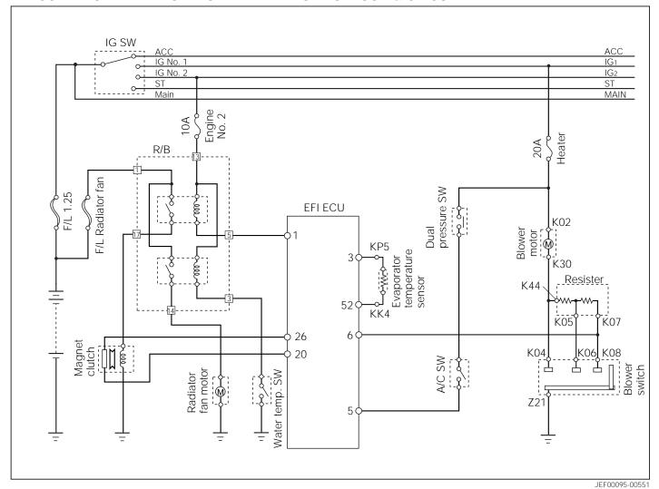
When the air conditioner evaporator temperature sensor and circuit becomes open or shorted:
