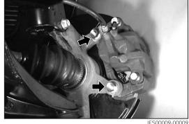
5. Remove the brake disc.
