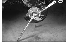
(3) Pull out the front axle hub sub-assembly with inner bearing race, using the following SST.
