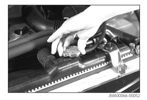
(27) Slowly pour a proper amount of antifreeze solution into the radiator in accordance with the instruction of the manufacturer of antifreeze solution.
