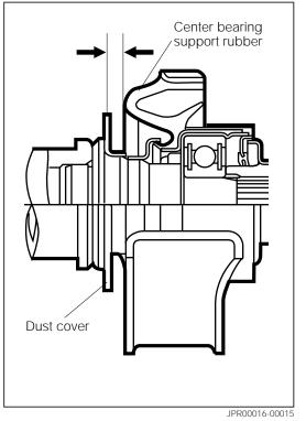
7. Ensure that the clearance between the center bearing support rubber and the dust cover is within the specified value.
