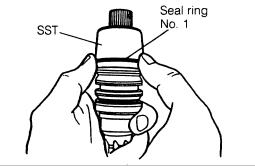
(3) Hold the seal rings attached to the control valve subassembly with your fingers and contract it so that the rings may be bedded in.
