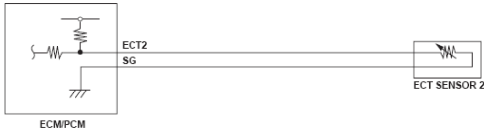
Fig. 226: Engine Coolant Temperature (ECT) Sensor 2 Circuit Diagram
