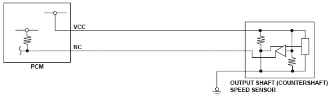
Fig. 108: Output Shaft (Countershaft) Speed Sensor Circuit Diagram
