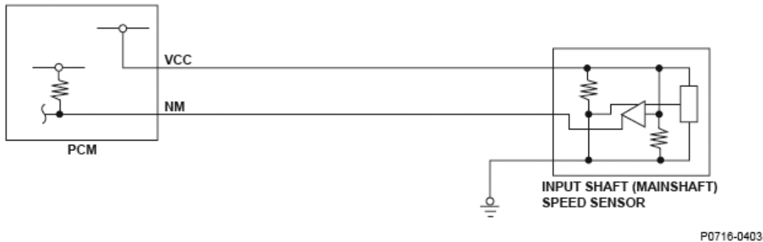
Fig. 101: Input Shaft (Mainshaft) Speed Sensor Circuit Diagram
