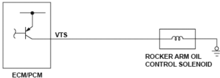
Fig. 247: Rocker Arm Oil Control Solenoid Circuit Diagram
