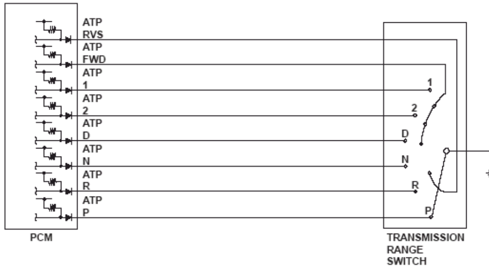
Fig. 202: Transmission Range Switch Circuit Diagram
