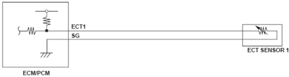
Fig. 18: Engine Coolant Temperature (ECT) Sensor 1 Circuit Diagram
