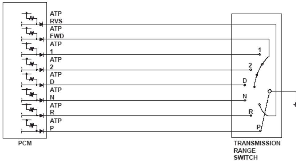
Fig. 91: Transmission Range Switch Circuit Diagram
