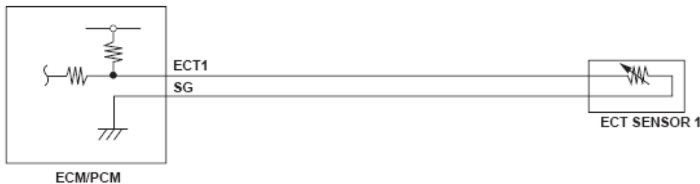
Fig. 20: Engine Coolant Temperature (ECT) Sensor 1 Circuit Diagram
