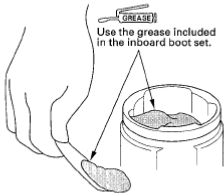
Fig. 88: Applying Grease On Inboard Boot Set Courtesy of TOYOTA MOTOR SALES, U.S.A., INC.
