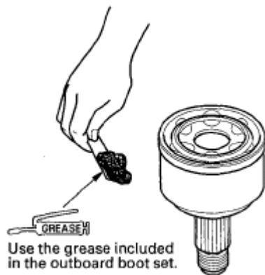
Fig. 42: Applying Grease On Outboard Joint Courtesy of TOYOTA MOTOR SALES, U.S.A., INC.
