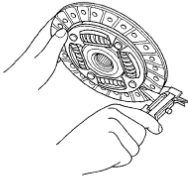
Fig. 26: Measuring Clutch Disc Thickness
