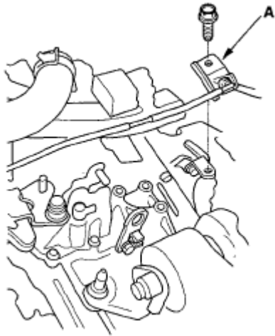
Fig. 17: Identifying Clutch Line Bracket Courtesy of AMERICAN HONDA MOTOR CO., INC.
