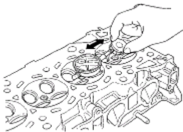
Fig. 105: Measuring Valve Stem-To-Guide Clearance Courtesy of AMERICAN HONDA MOTOR CO., INC.
