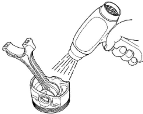
Fig. 34: Heating Piston And Connecting Rod Assembly Courtesy of AMERICAN HONDA MOTOR CO., INC.
