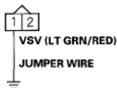
Fig. 33: Connecting EVAP Canister Vent Shut Valve 2P Connector Terminal No. 1 To Body Ground With Jumper Wire
