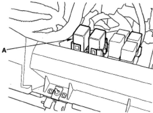
Fig. 24: Identifying PGM-FI Main Relay 2 (FUEL PUMP) Courtesy of AMERICAN HONDA MOTOR CO., INC.
