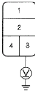
Fig. 52: Measuring Voltage Between No. 3 Terminal Of A/C Compressor Clutch Relay 4P Socket And Body Ground
