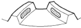
Fig. 212: Identifying Correct Tooth Contact Pattern Courtesy of AMERICAN HONDA MOTOR CO., INC.
