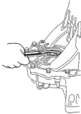
Fig. 170: Measuring Clearance Between Shim And Bearing Outer Race In Transmission Housing Courtesy of AMERICAN HONDA MOTOR CO., INC.
