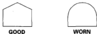
Fig. 121: Identifying Example Of Synchro Ring Teeth Courtesy of AMERICAN HONDA MOTOR CO., INC.
