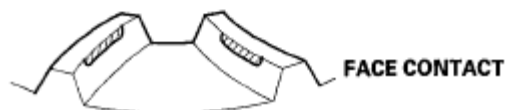
Fig. 213: Identifying Incorrect Tooth Contact Pattern Courtesy of AMERICAN HONDA MOTOR CO., INC.
