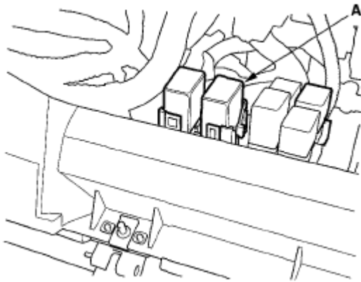
Fig. 85: Identifying PGM-FI Main Relay 1 (FI MAIN)
