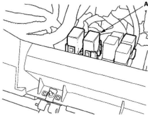
Fig. 81: Identifying PGM-FI Main Relay 1 (FI MAIN) Courtesy of AMERICAN HONDA MOTOR CO., INC.
