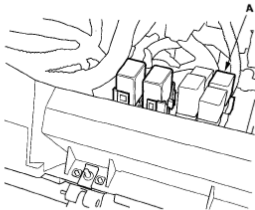
Fig. 37: Identifying A/F Sensor Relay (LAF) Courtesy of AMERICAN HONDA MOTOR CO., INC.
