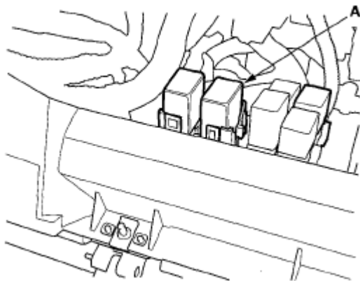
Fig. 157: Identifying PGM-FI Main Relay 1 (FI MAIN) Courtesy of AMERICAN HONDA MOTOR CO., INC.
