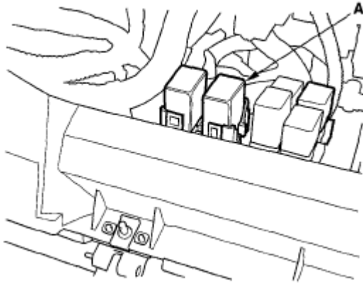
Fig. 148: Identifying PGM-FI Main Relay 1 (FI MAIN) Courtesy of AMERICAN HONDA MOTOR CO., INC.
