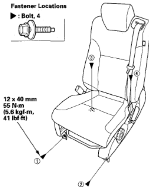
Fig. 7: Removal/Installation Of Front Seat With Torque Specification Courtesy of AMERICAN HONDA MOTOR CO., INC.
