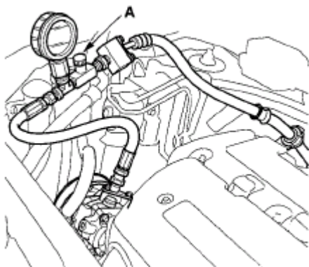
Fig. 9: Identifying Pressure Control Valve
