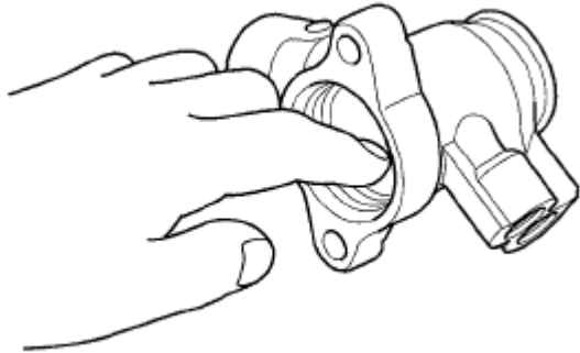
Fig. 87: Checking Inner Wall Of Valve Housing Where Seal Ring Slides Courtesy of AMERICAN HONDA MOTOR CO., INC.
