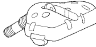
Fig. 15: Identifying Control Unit And Tire Pressure Sensor Courtesy of AMERICAN HONDA MOTOR CO., INC.
