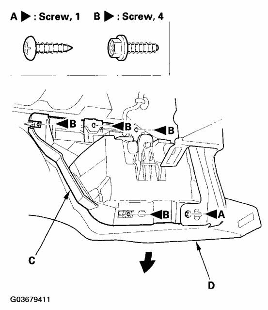
Fig. 5: Removing Screws From Under Dashboard Courtesy of AMERICAN HONDA MOTOR CO., INC.
