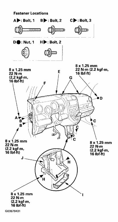
Fig. 25: Detaching Harness And Connector Clips And Torque Specifications Courtesy of AMERICAN HONDA MOTOR CO., INC.
