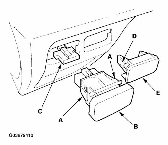
Fig. 4: Disconnecting Connector By Releasing Cruise Control Main Switch Courtesy of AMERICAN HONDA MOTOR CO., INC.
