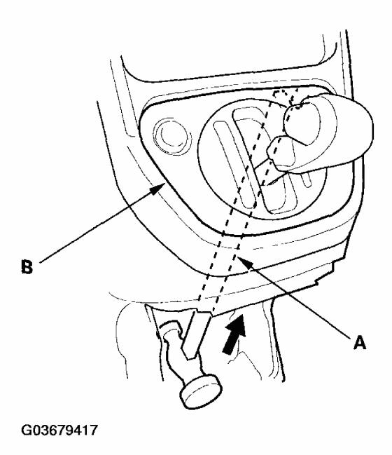
Fig. 11: Inserting Handle Through Center Lower Cover To Shift Lever Trim Courtesy of AMERICAN HONDA MOTOR CO., INC.
