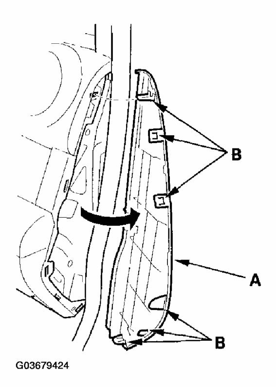
Fig. 18: Pulling Front Of Dashboard Side Lid Courtesy of AMERICAN HONDA MOTOR CO., INC.
