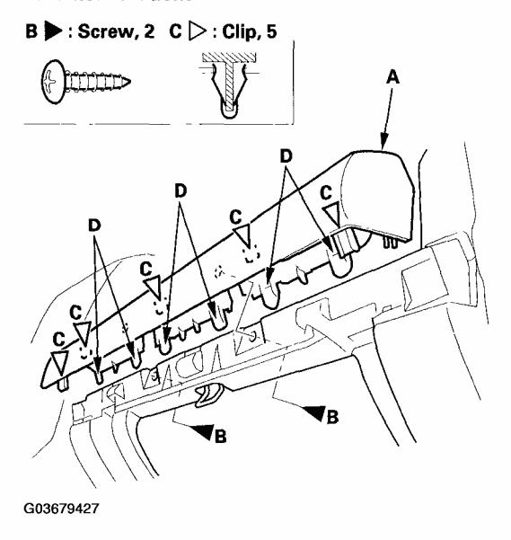
Fig. 21: Removing Dashboard Lower Panel Courtesy of AMERICAN HONDA MOTOR CO., INC.
