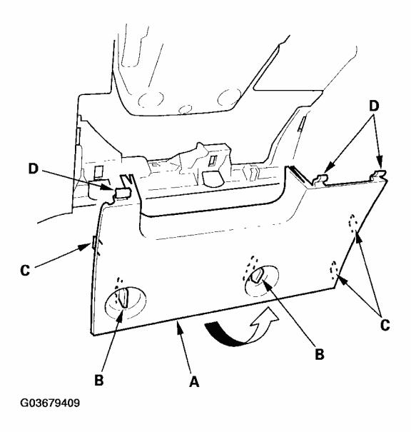
Fig. 3: Removing Driver's Dashboard Lower Cover Courtesy of AMERICAN HONDA MOTOR CO., INC.
