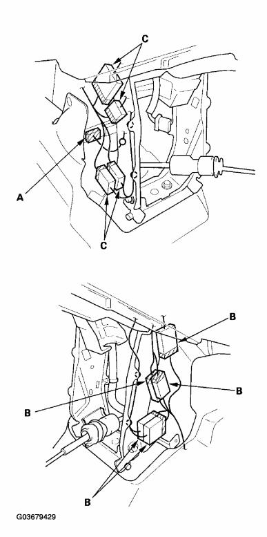
Fig. 23: Disconnecting SRS Control Unit Connector Courtesy of AMERICAN HONDA MOTOR CO., INC.
