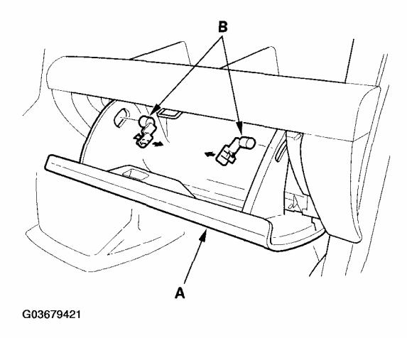
Fig. 15: Removing Glove Box Stop Courtesy of AMERICAN HONDA MOTOR CO., INC.
