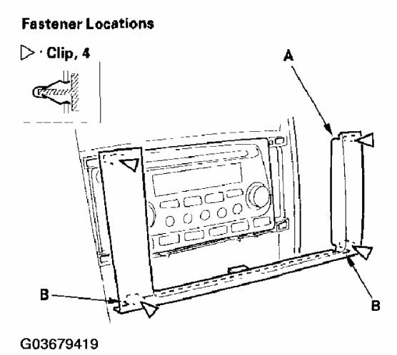
Fig. 13: Releasing Lower Clips In Radio Panel Courtesy of AMERICAN HONDA MOTOR CO., INC.
