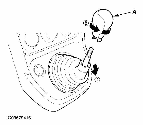
Fig. 10: Removing Shift Knob Courtesy of AMERICAN HONDA MOTOR CO., INC.
