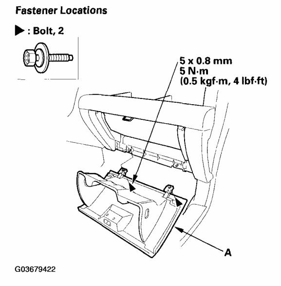
Fig. 16: Removing Glove Box Bolt With Specified Torques Courtesy of AMERICAN HONDA MOTOR CO., INC.
