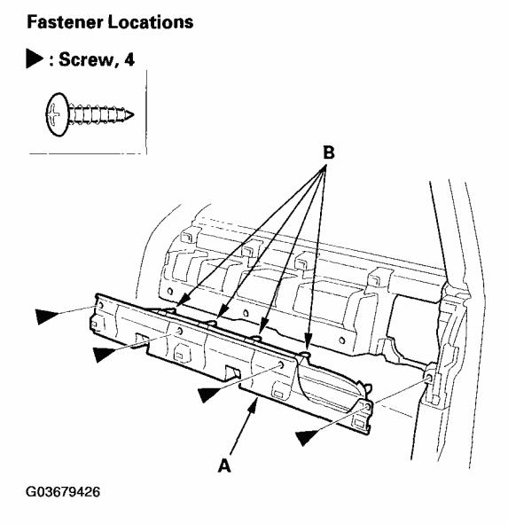
Fig. 20: Removing Dashboard Tray Cover Courtesy of AMERICAN HONDA MOTOR CO., INC.
