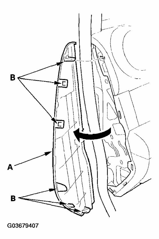
Fig. 1: Removing Dashboard Side Lid
