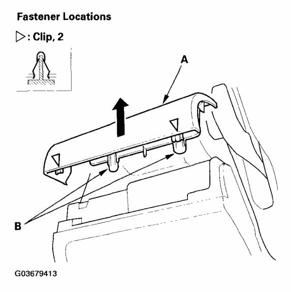
Fig. 7: Pulling Driver's Outer Dashboard Trim Courtesy of AMERICAN HONDA MOTOR CO., INC.
