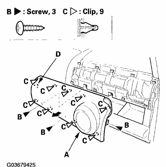
Fig. 19: Removing Dashboard Upper Panel Courtesy of AMERICAN HONDA MOTOR CO., INC.
