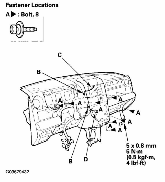
Fig. 26: Detaching Harness Clips And Torque Specifications Courtesy of AMERICAN HONDA MOTOR CO., INC.
