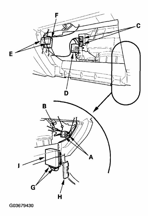
Fig. 24: Disconnecting Passenger' Door Wire Harness Connectors Courtesy of AMERICAN HONDA MOTOR CO., INC.
