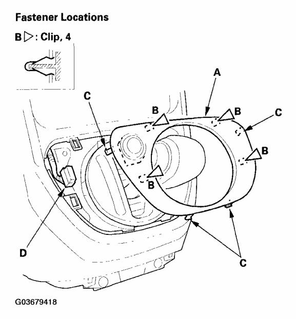
Fig. 12: Pulling Shift Lever Trim Releasing Clips & Hooks. Courtesy of AMERICAN HONDA MOTOR CO., INC.
