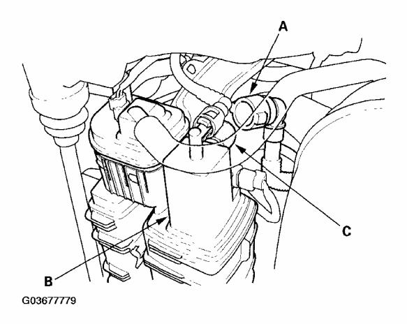
Fig. 3: Disconnecting Fuel Tank Vapor Recirculation Tube From EVAP Canister Courtesy of AMERICAN HONDA MOTOR CO., INC.
