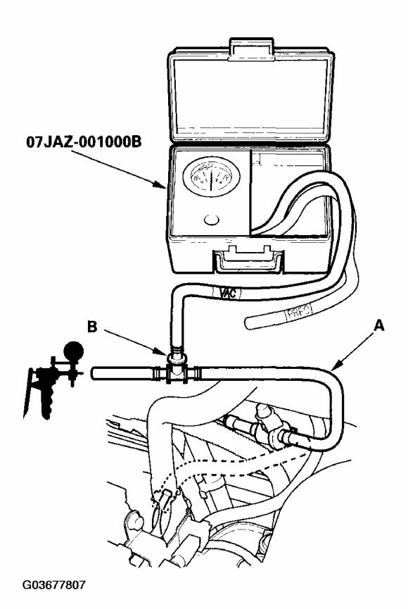
Fig. 31: Disconnecting Vacuum Hose From EVAP Canister Purge Line
