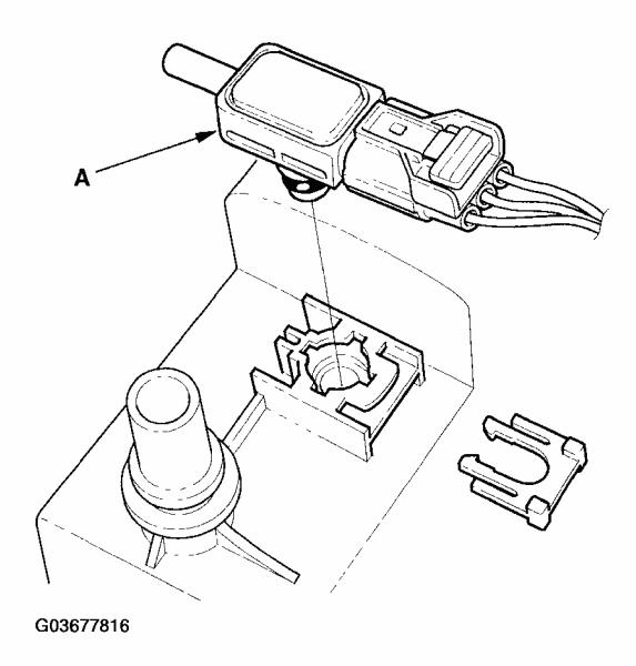
Fig. 40: Removing FTP Sensor From EVAP Canister Courtesy of AMERICAN HONDA MOTOR CO., INC.
