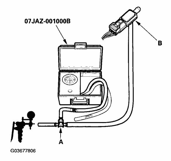
Fig. 30: Connecting T-Fitting From Vacuum Gauge And Vacuum Pump To FTP sensor
