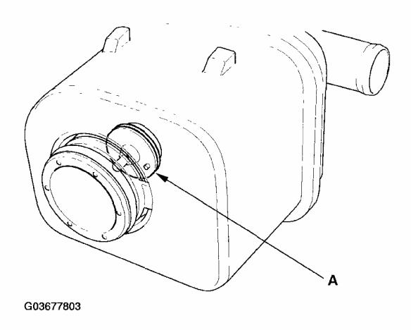
Fig. 27: Identifying EVAP Canister Vent Shut Valve Courtesy of AMERICAN HONDA MOTOR CO., INC.
