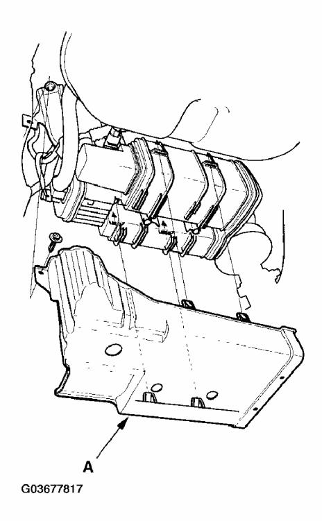
Fig. 41: Removing EVAP Canister Cover Courtesy of AMERICAN HONDA MOTOR CO., INC.
