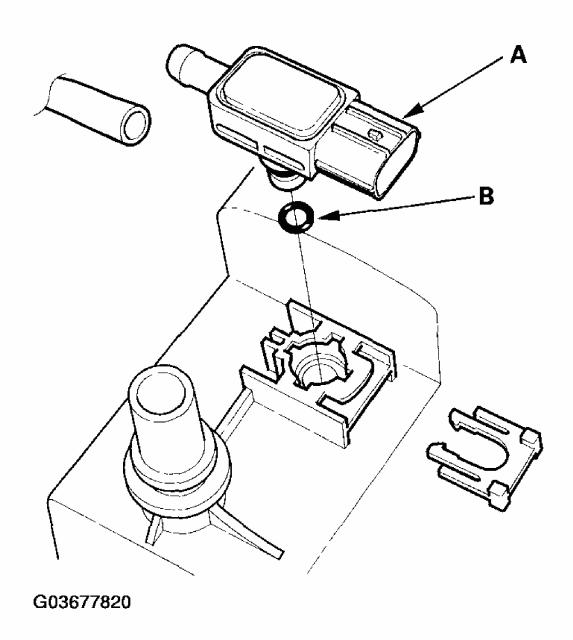
Fig. 44: Removing FTP Sensor Courtesy of AMERICAN HONDA MOTOR CO., INC.
