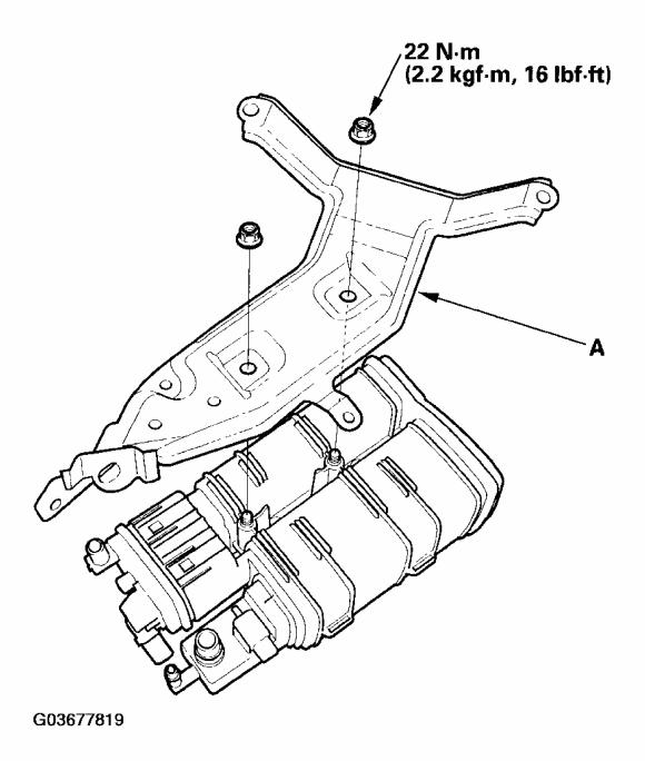
Fig. 43: Removing EVAP Canister Bracket And Torque Specifications Courtesy of AMERICAN HONDA MOTOR CO., INC.
