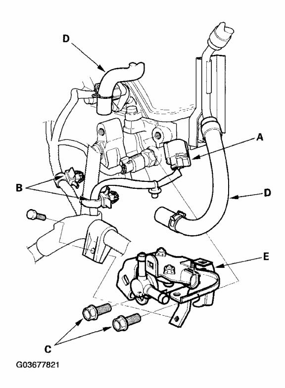
Fig. 45: Disconnecting EVAP Canister Purge Valve 2P Connector Courtesy of AMERICAN HONDA MOTOR CO., INC.
