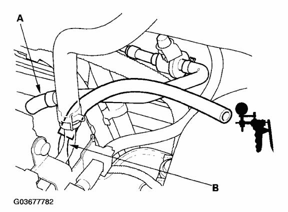
Fig. 6: Disconnecting Vacuum Hose From EVAP Canister Purge Valve In Engine Compartment
