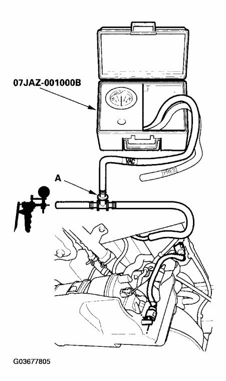
Fig. 29: Connecting T-Fitting From Vacuum Gauge And Vacuum Pump To EVAP Canister Purge Valve (2 Of 2)
