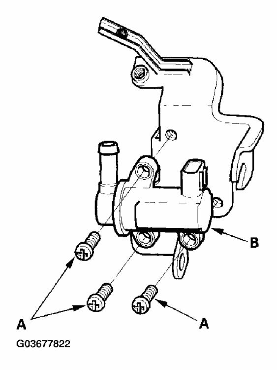
Fig. 46: Removing EVAP Canister Purge Valve From Bracket Courtesy of AMERICAN HONDA MOTOR CO., INC.
