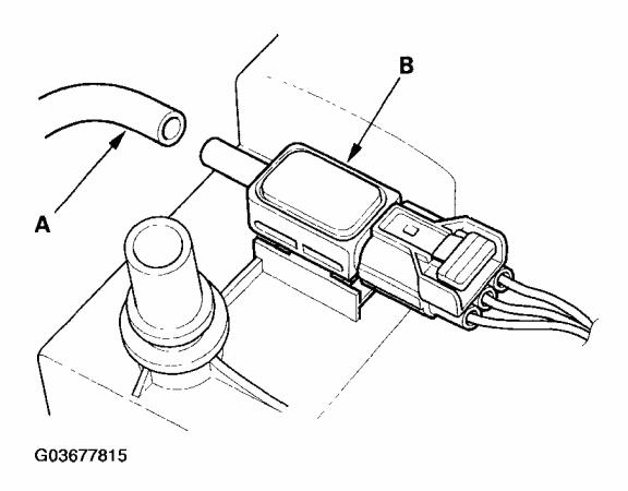
Fig. 39: Disconnecting Air Tube From FTP Sensor Courtesy of AMERICAN HONDA MOTOR CO., INC.
