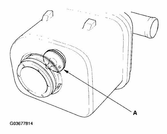
Fig. 38: Identifying EVAP Canister Vent Shut Valve Courtesy of AMERICAN HONDA MOTOR CO., INC.
