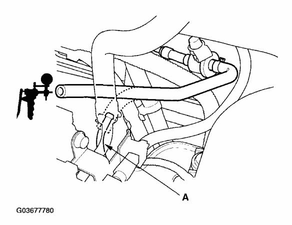
Fig. 4: Disconnecting Vacuum Hose From EVAP Canister Purge Valve And Connecting Vacuum Gauge
