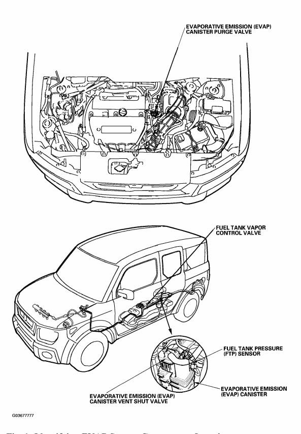
Fig. 1: Identifying EVAP System Components Location Courtesy of AMERICAN HONDA MOTOR CO., INC.
