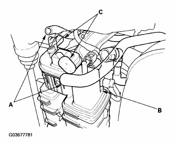
Fig. 5: Disconnecting Purge Air Hoses From EVAP Canister Vent Shut Valve Courtesy of AMERICAN HONDA MOTOR CO., INC.
