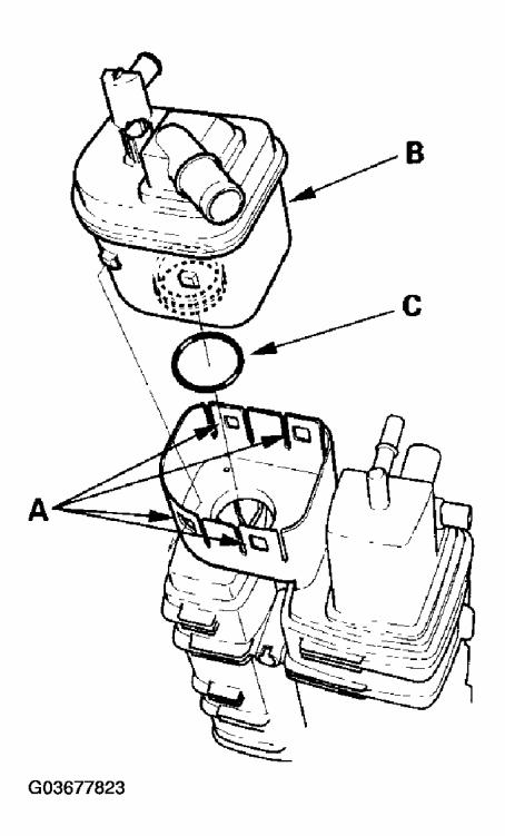
Fig. 47: Removing EVAP Canister Vent Shut Valve Courtesy of AMERICAN HONDA MOTOR CO., INC.
