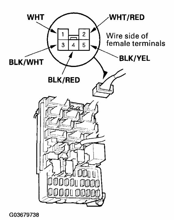
Fig. 1: Disconnecting Connector A (5P) From Under-Dash Fuse/Relay Box Courtesy of AMERICAN HONDA MOTOR CO., INC.
