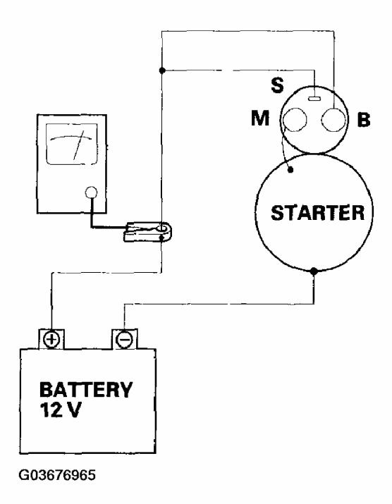
Fig. 12: Connecting Starter To Battery
