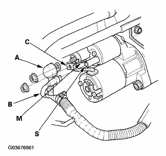
Fig. 8: Removing Starter Cable Courtesy of AMERICAN HONDA MOTOR CO., INC.
