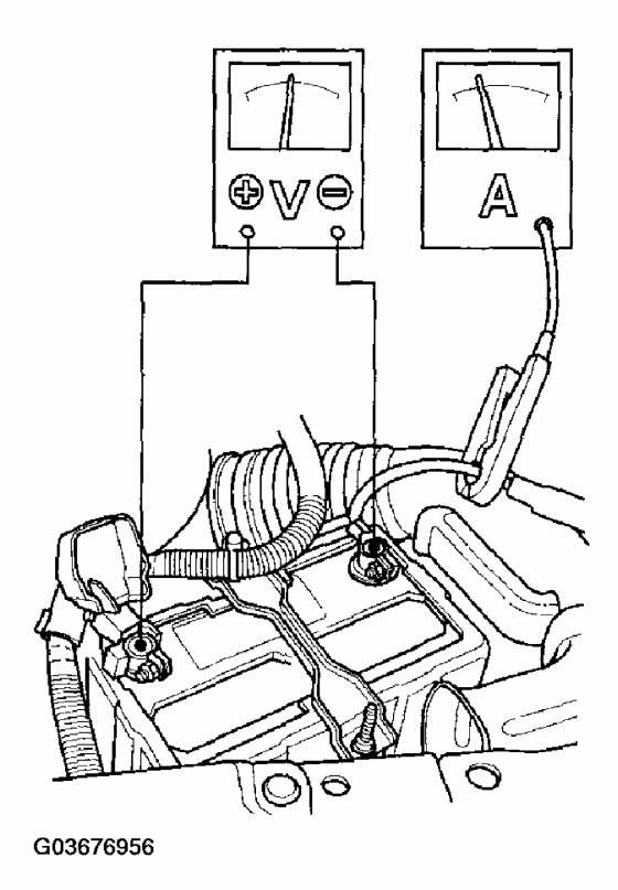
Fig. 3: Hooking Up Ammeter And Voltmeter Courtesy of AMERICAN HONDA MOTOR CO., INC.
