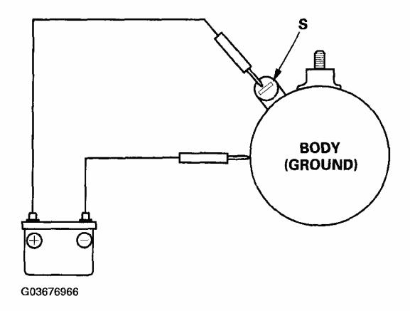
Fig. 13: Connecting Battery To Starter
