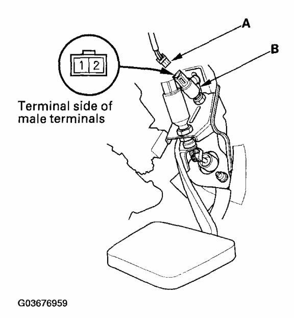
Fig. 6: Disconnecting Clutch Interlock Switch 2P Connector Courtesy of AMERICAN HONDA MOTOR CO., INC.
