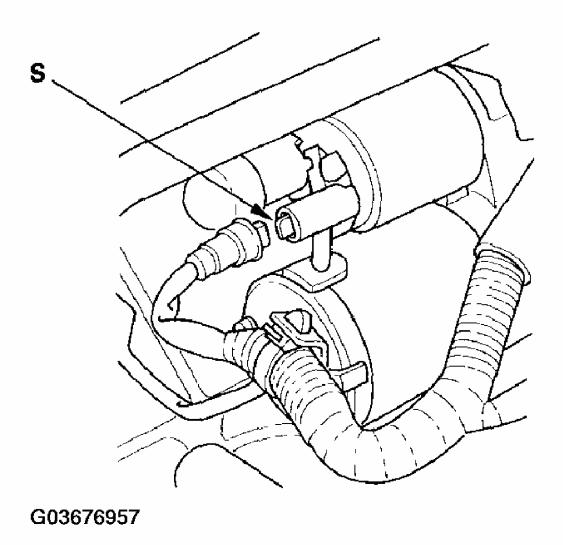
Fig. 4: Disconnecting BLK/WHT Wire From Starter Solenoid S Terminal (M/T) Courtesy of AMERICAN HONDA MOTOR CO., INC.
