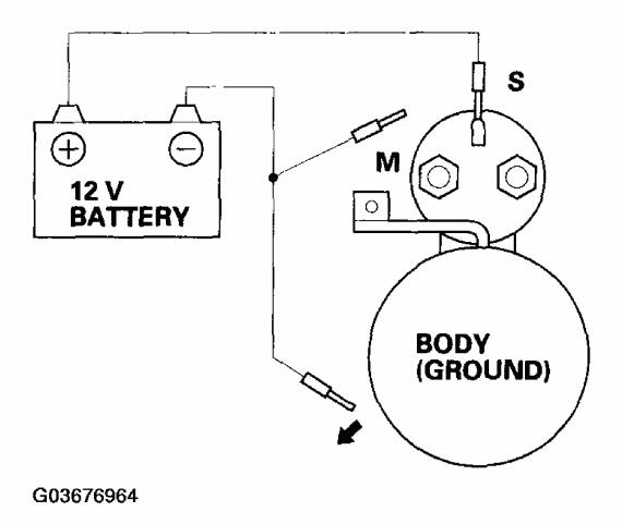
Fig. 11: Disconnecting Negative Battery Terminal From Starter Body Courtesy of AMERICAN HONDA MOTOR CO., INC.
