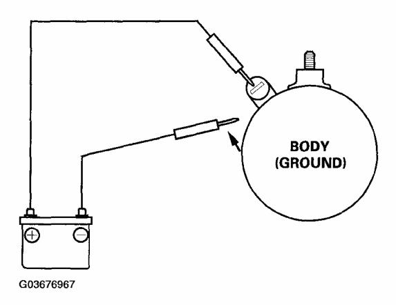
Fig. 14: Disconnecting Negative Battery Terminal From Starter Courtesy of AMERICAN HONDA MOTOR CO., INC.
