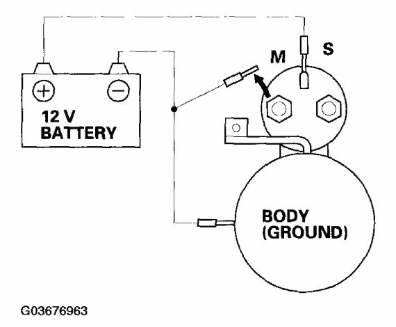
Fig. 10: Disconnecting Negative Battery Terminal From M Terminal Courtesy of AMERICAN HONDA MOTOR CO., INC.
