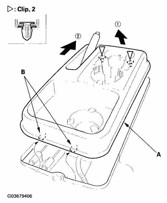
Fig. 1: Removing Center Console
