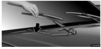
To return the windshield wipers to retracted position, push the connection of the wiper arm and wiper blade downward.
