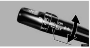
To turn on the fog lights, turn the switch to the "ON" position. The fog lights come on only when the headlights are on low beam.
