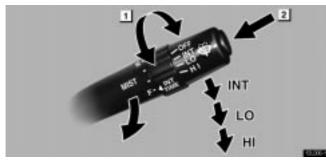
▶ 1 Interval adjuster 2 Washer on
