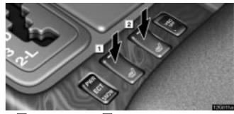
▶ 1 For driver's seat 2 For front passenger's seat
