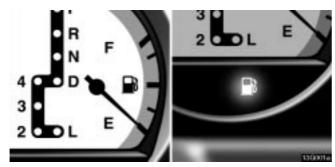
The gauge is displayed when the ignition switch is on and indicates the approximate quantity of fuel remaining in the tank.
