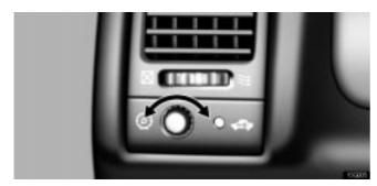
The brightness of the instrument panel lights is automatically adjusted depending on the brightness of your surroundings. To adjust the brightness as you like, turn the knob. However, if the brightness is automatically adjusted at the maximum, turning the knob cannot change the brightness.
