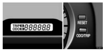
This meter displays the odometer and two trip meters. To change the mode indication, push the "ODO/TRIP" button.
