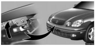
2. Insert your fingers under the hood, push up the auxiliary catch lever and lift the hood.
