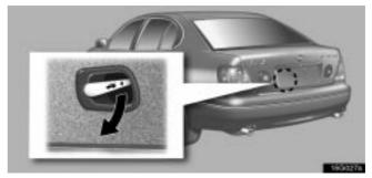
If a person is locked in the trunk, pull down the phosphorescent handle (illuminated for a while) on the inside of trunk lid in case of emergency to open the trunk lid.
