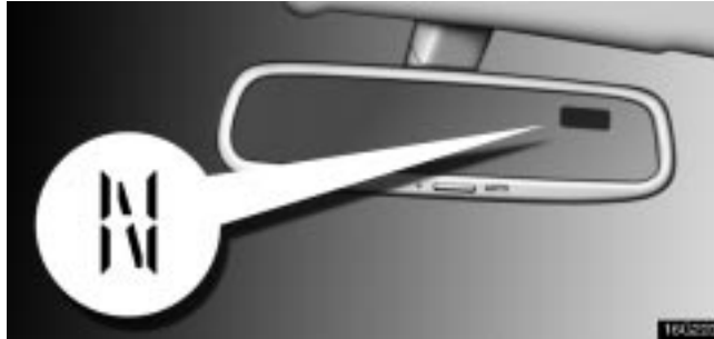
The compass indicates the direction in which the vehicle is heading. The illustration shown above indicates the vehicle is heading north.
