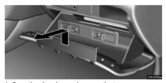
1. Open the glove box and remove the two covers.
