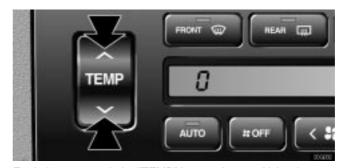
Each time you push the "TEMP" button, the sensitivity changes from "+3" down to "-3". If you do not operate any button for a few seconds or if you push the button other than the air intake control button and driver side temperature control button, the previous display returns.
