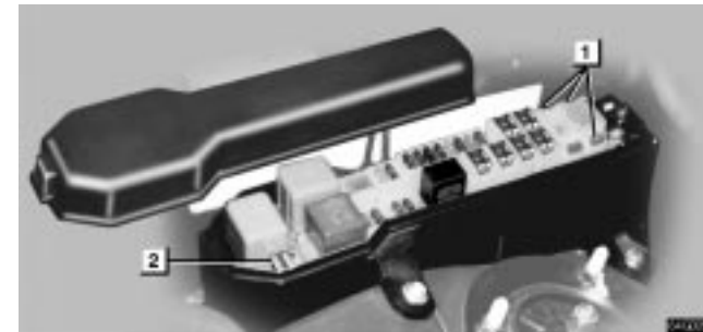
► Engine compartment 1 Spare fuses 2 Pull-out tool
