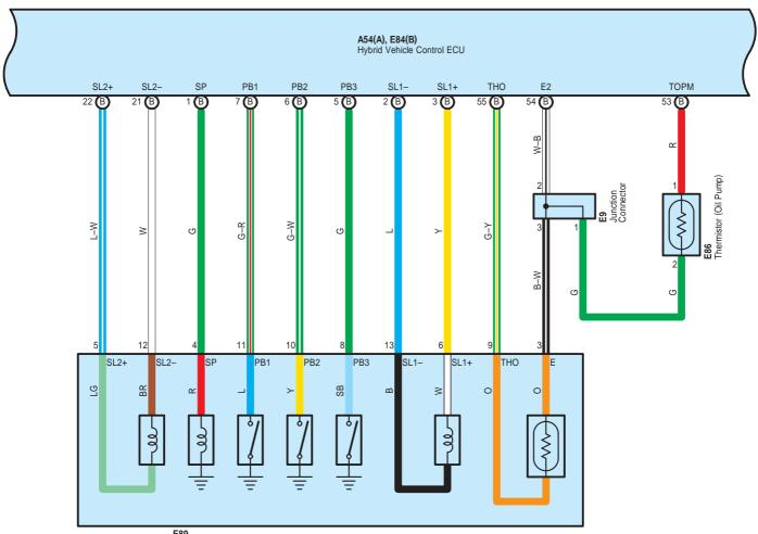
E89 Electronically Controlled Transmission Solenoid
